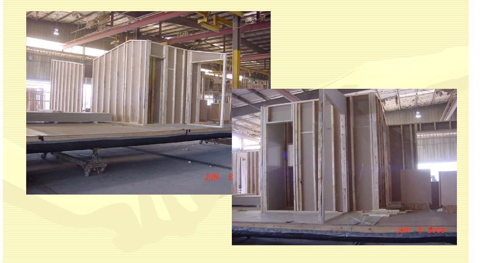
FLOORS, WALLS AND CEILING ARE SECURELY FASTENED WITH GALVENIZED METAL STRAPS.
